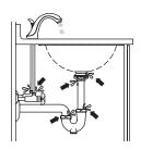
Run water into the lavatory and check for leaks.
